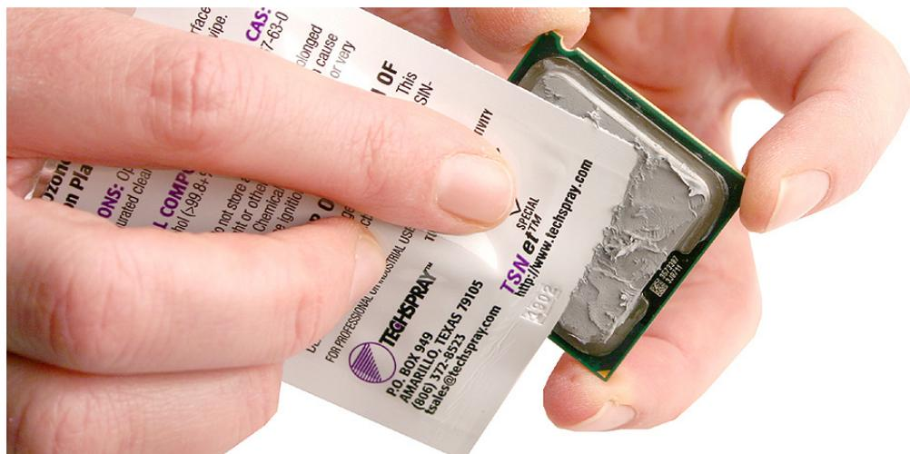
3. Holding the processor by three corners only, keep the processor level as you place it into its holder on the logic board, being careful not to get any thermal grease on the contacts of either the processor or its socket holder.
