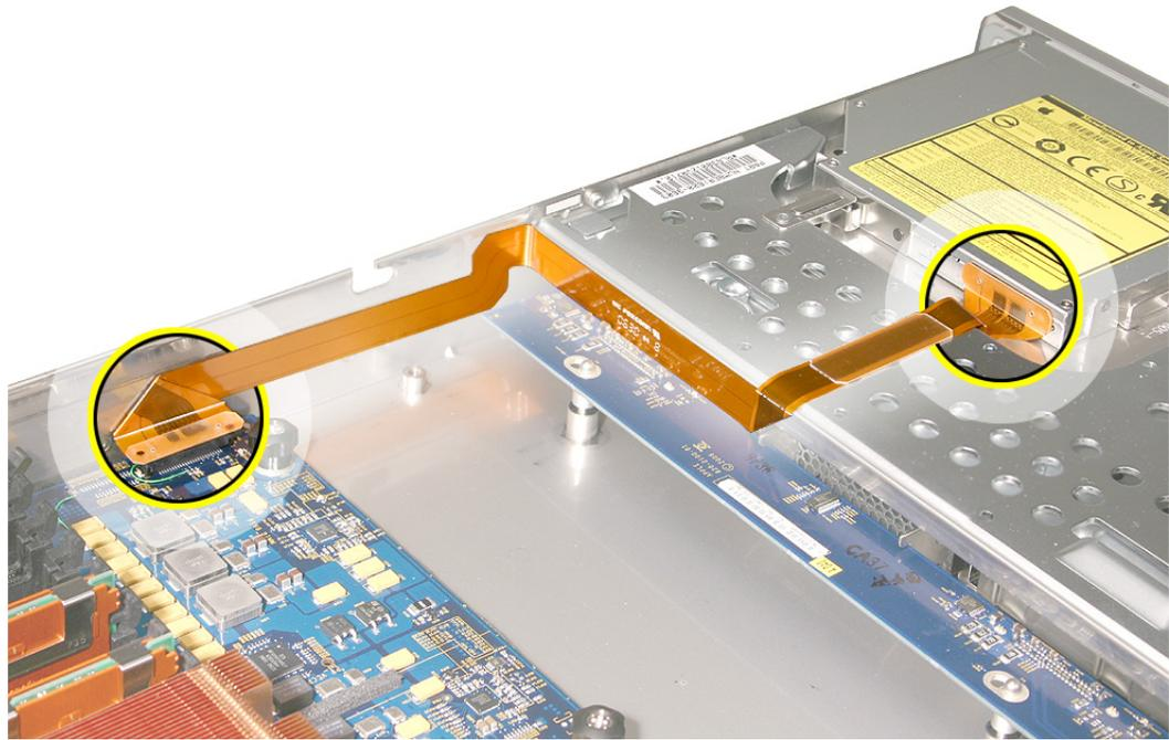
3. Carefully pry the cable's adhesive from the enclosure and remove the cable from the Xserve.
