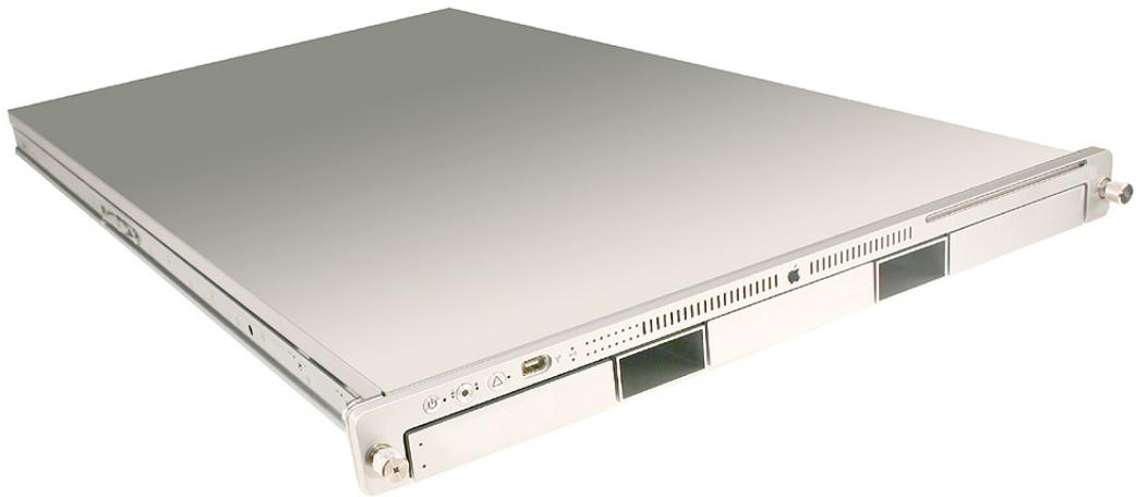
The only noticeable external difference between the Xserve (Late 2006) model and the Xserve (Early 2008) model is the port next to the system identifier button on the front bezel. On the Xserve (Late 2006) model, it is a FireWire 400 port; whereas on the Xserve (Early 2008) model, it is a USB port, as shown below.
