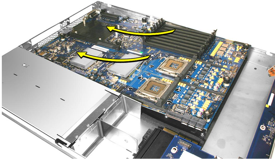
**Replacement Note:** Remove the battery insulator tab from the battery holder on the replacement logic board. Depending on the Xserve model, the battery position may differ from what is shown.
