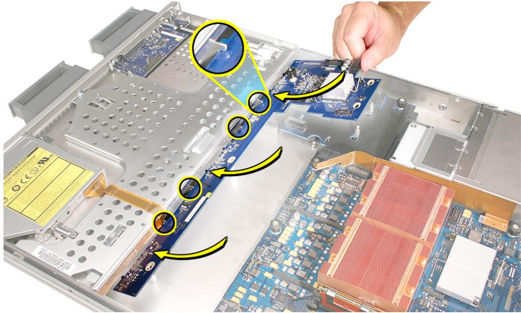
Then rotate the backplane downward and over the four mushroom-shaped standoffs. Finally, slide the backplane in the direction of the arrow shown to fully seat the backplane in the enclosure.
