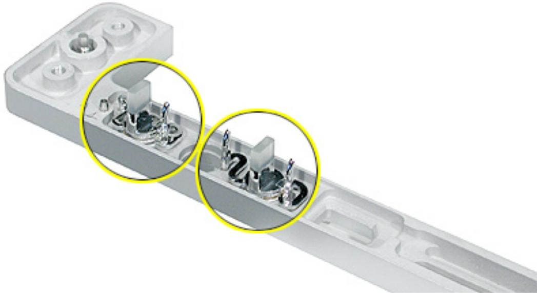
2. Position the light pipes in the light pipe assembly into the double row of light pipe holes in the front bezel.
