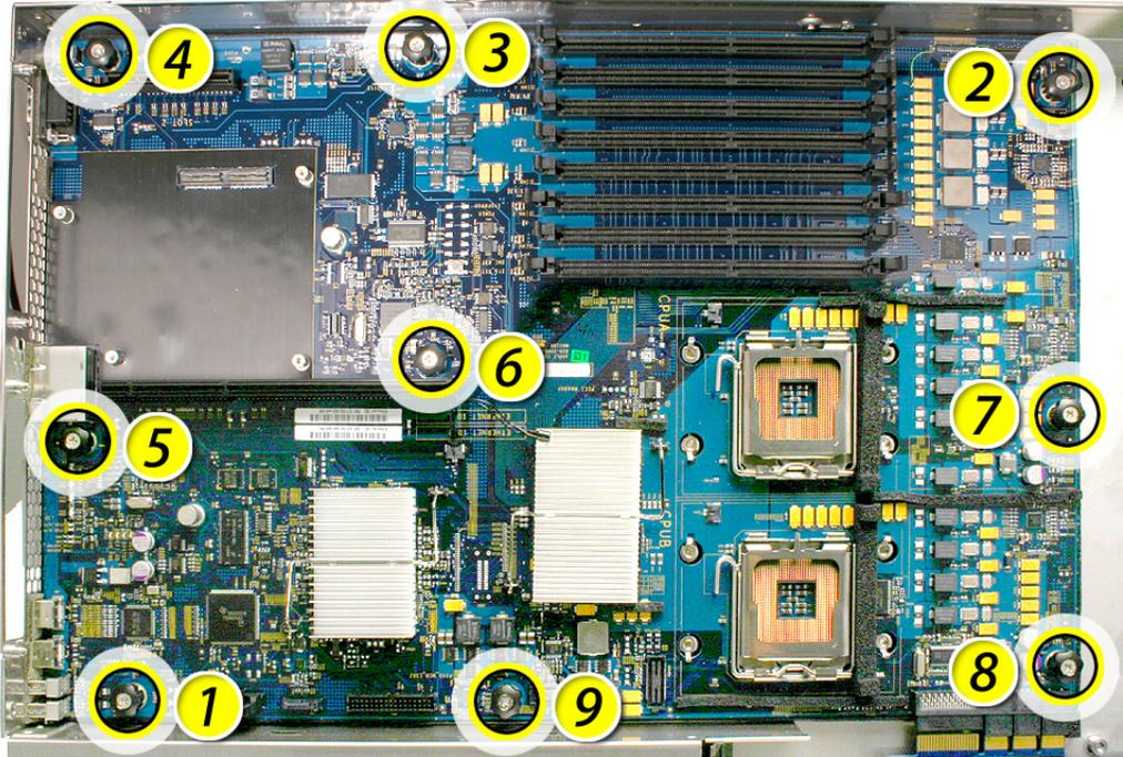
6. Grasping the logic board only by its expansion card riser and edge as shown, move it forward and up slightly to release it from the rear port openings in the enclosure.
