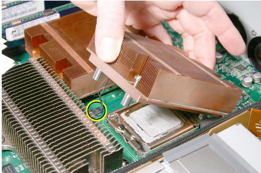
4. Lift the heat sink straight up and out of the enclosure.
