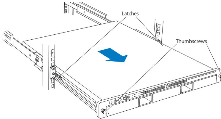
6. When the safety latches engage, grip the Xserve where it emerges from the rack, press down on the latch tabs with your thumbs, and slide the Xserve the rest of the way out of the rack rails. Set the Xserve on a flat surface.
