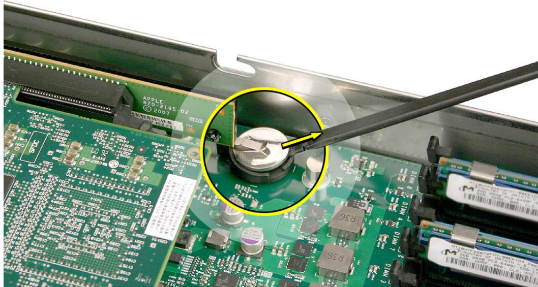
2. Insert the replacement battery in the holder with the positive side (+) up and the negative side down.
