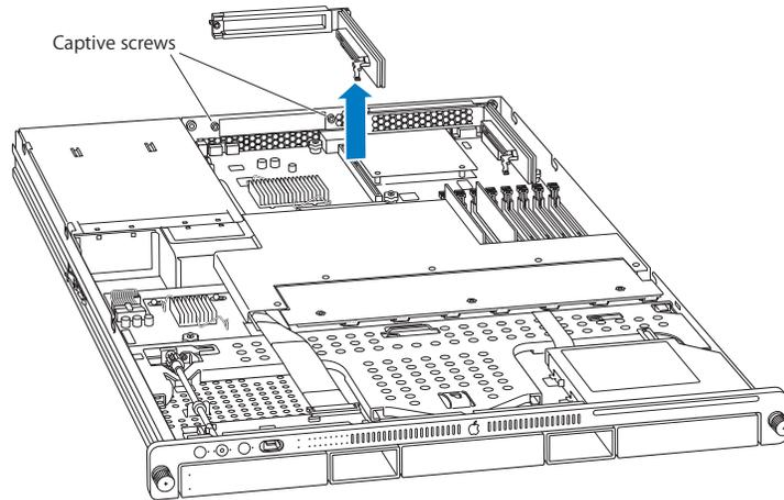
2. Carefully pull up on the bracket and riser, to disconnect the riser from the logic board. If you are removing a blank riser card so that you can install a graphics card in the riser, do the following:
