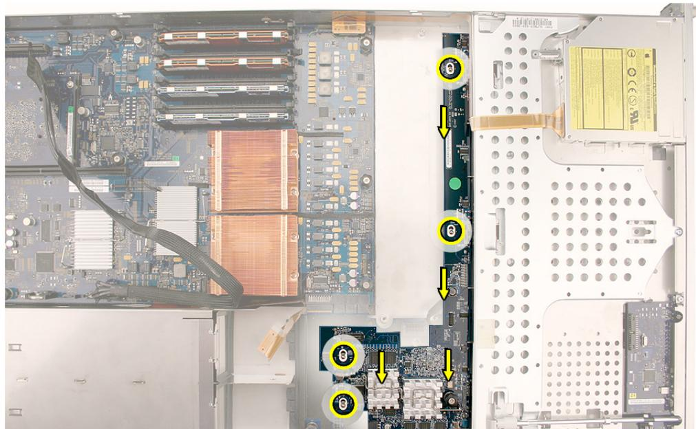
6. Rotate the Xserve RAID Card up slightly from the logic board side (as shown), and carefully pull the card up and toward the logic board to free it from the standoffs and four alignment slots in the enclosure. Be careful not to let any Xserve RAID Card components come into contact with the standoffs or the enclosure as you remove the card.
