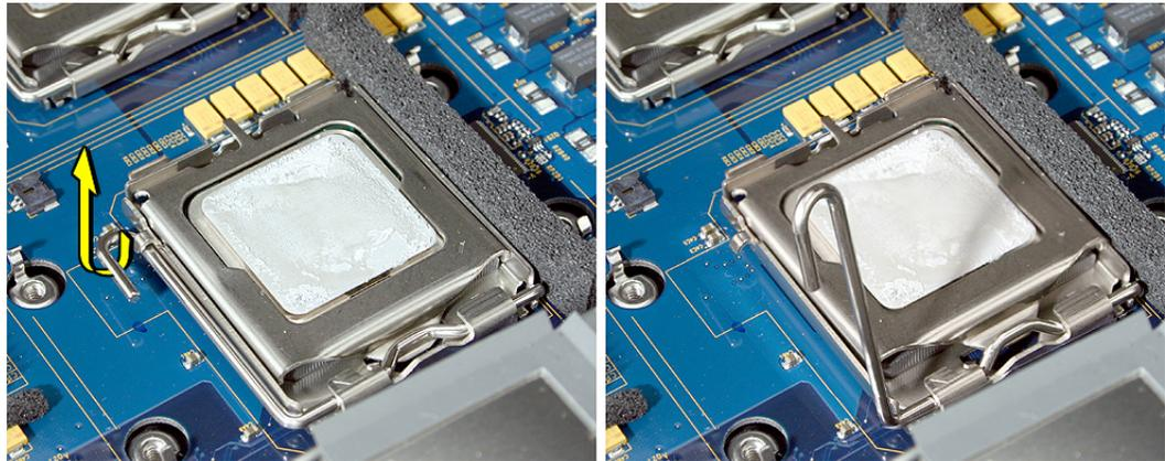
3. Carefully lift the processor out of the holder.
