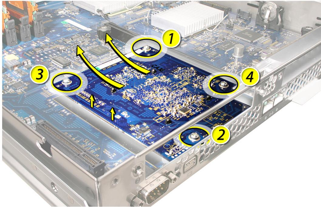
**Replacement Note:** When installing the mezzanine card, be sure to press down gently and evenly on it to seat the connector on the underside of the card to the logic board. Then replace the four screws, and secure them in the order shown above.
