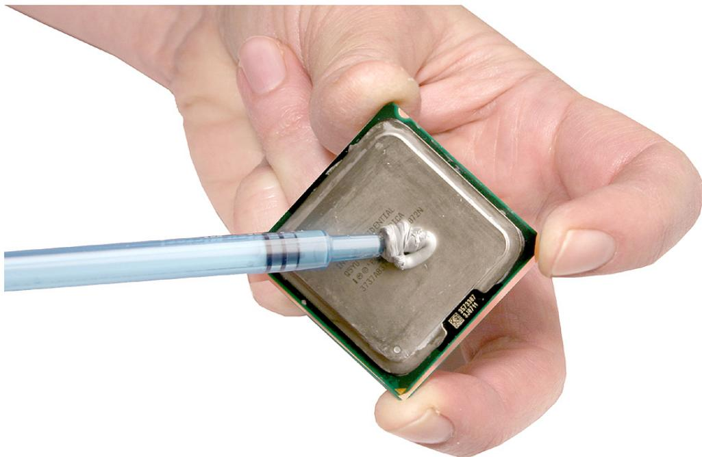
6. Use the edge of the package that the alcohol wipe came in as a spatula to spread the thermal grease evenly over the entire top surface of the processor. Scrape off any excess grease with the package edge, then discard the package.
