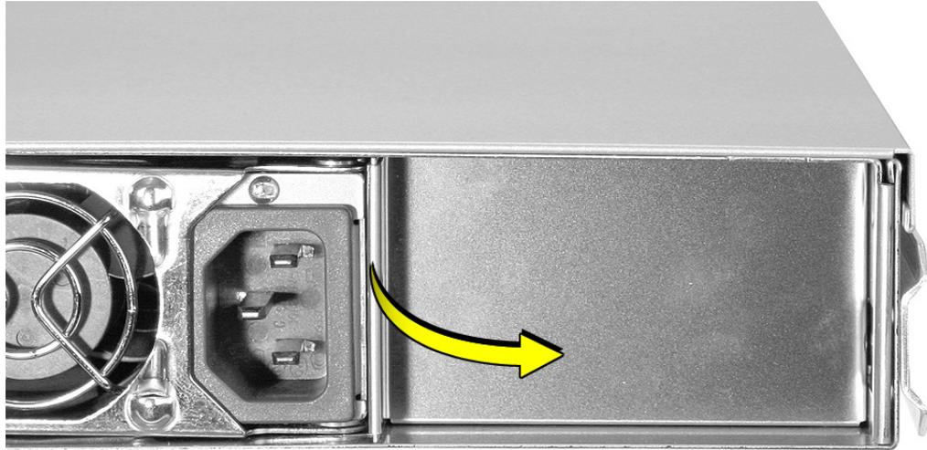
2. Notice the hook that catches on the inside bottom of the power supply bay.
