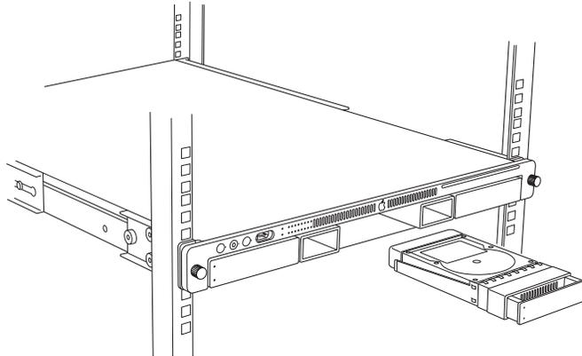
You can replace or install hard drives while the Xserve is running; you do not need to shut down or open the Xserve first, but you may need to dismount the drive from the Xserve OS beforehand. A status light on the front of each drive indicates when it is safe to remove the drive without losing data. For more information, see “Hard Drive Module” in the Take Apart chapter.
