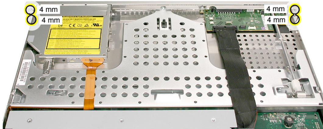
**Important:** When removing or replacing the bezel brackets, be careful not to put pressure on the top of the bezel over the optical drive slot.
