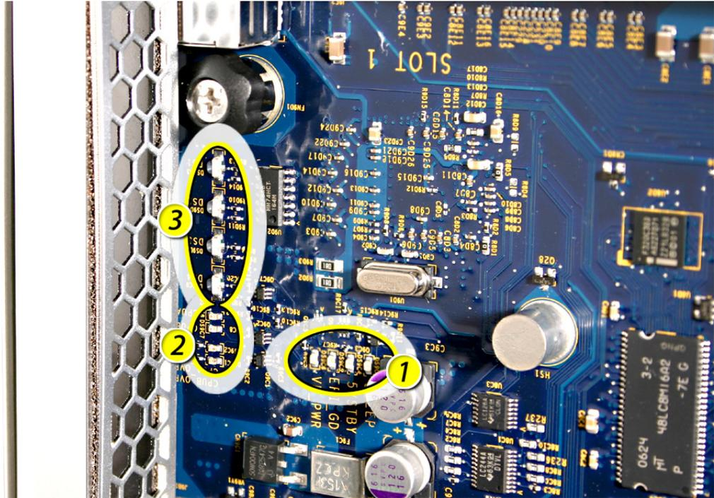
The LEDs are located toward the rear of the logic board. You must remove the top cover of the Xserve for the diagnostic LEDs to function.
