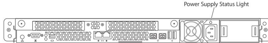
If the Xserve is already running when inserting a second power supply, the status light on the new supply will illuminate SOLID GREEN when it's turned on, to indicate normal operation as it starts sharing the load.
