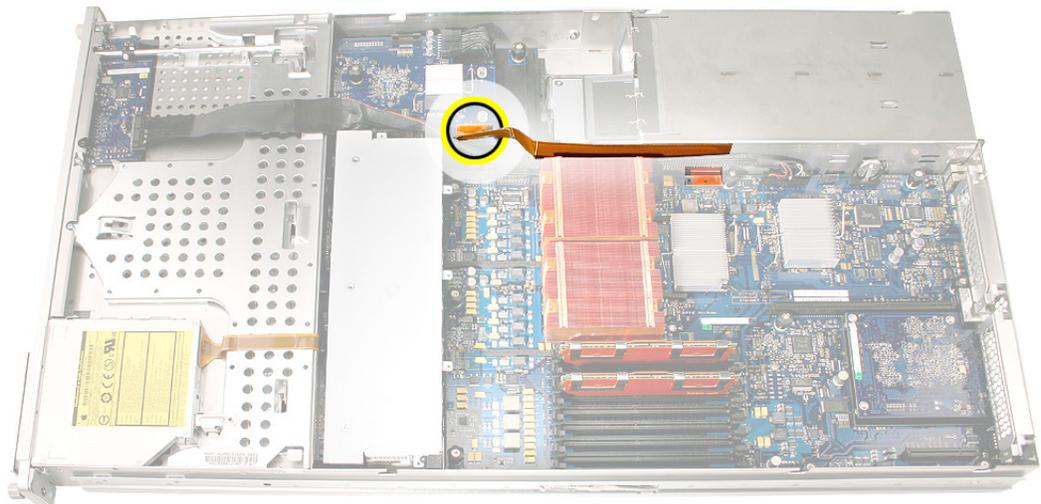
**Replacement Note:** Before installing the cable, fold it to a 90-degree angle along its creases.
