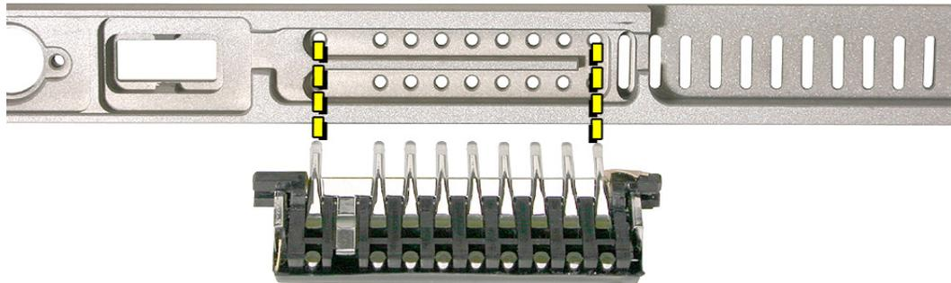
3. Replace the front bezel on the server, matching ports/projections with openings.
