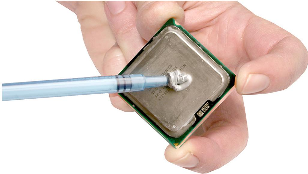
2. Use the edge of the package that the alcohol wipe came in as a spatula to spread the thermal grease evenly over the entire top surface of the processor. Scrape off any excess grease with the package edge, then discard the package.
