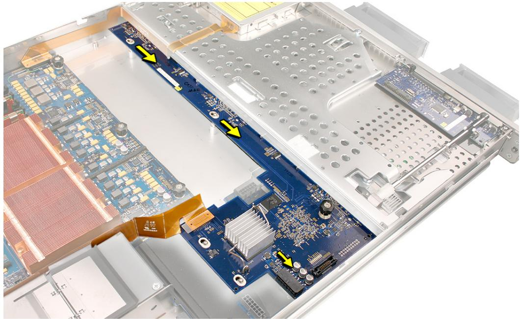
5. Rotate the backplane up slightly from the logic board side (as shown), and carefully pull the backplane up and toward the logic board to free it from the standoffs and four backplane alignment slots in the enclosure. Be careful not to let any backplane components come into contact with the standoffs or the enclosure as you remove the backplane.
