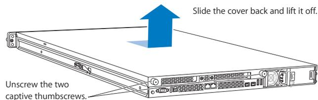
8. When you're finished working inside the Xserve, replace and secure the cover, slide the Xserve back into the rack, and tighten the front thumbscrews to secure the Xserve in the rack. If the server case was locked, use the enclosure key to lock the security lock on the front panel.
