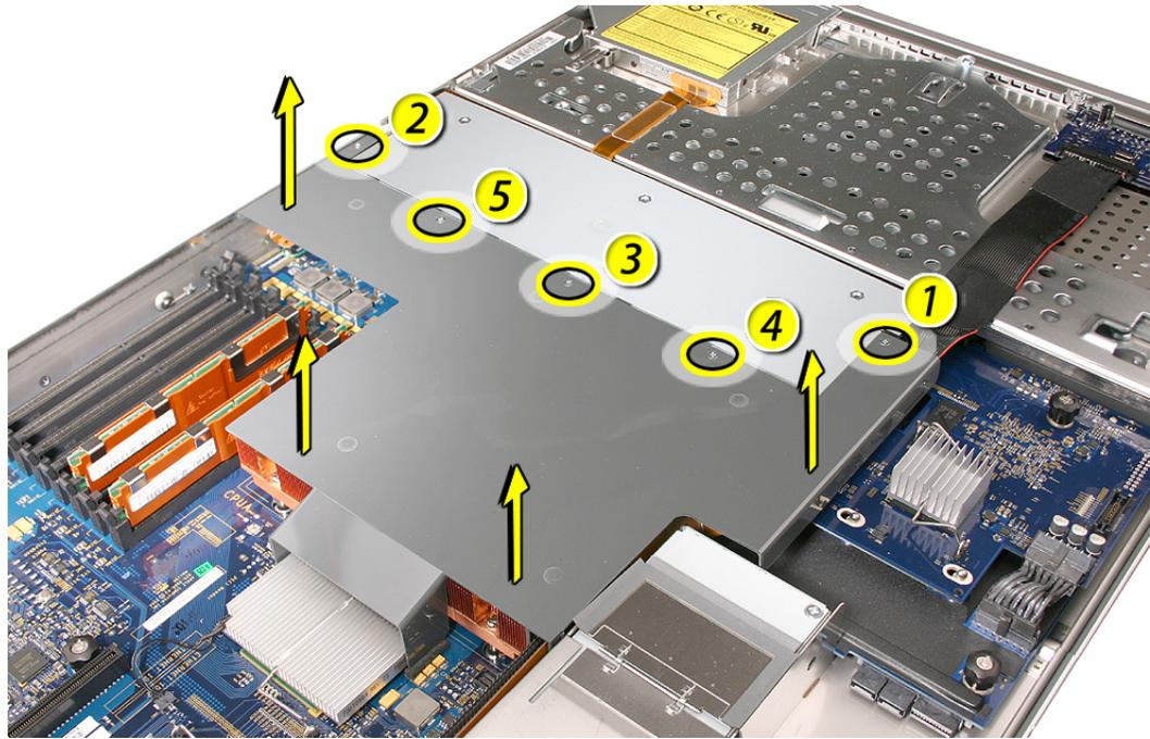
**Caution:** Try not to completely remove the screws from the airflow duct. Tiny black rubber washers hold these screws captive on the underside of the airflow duct. If the screws are completely removed, these rubber washers can easily fall into the enclosure and become lost.
