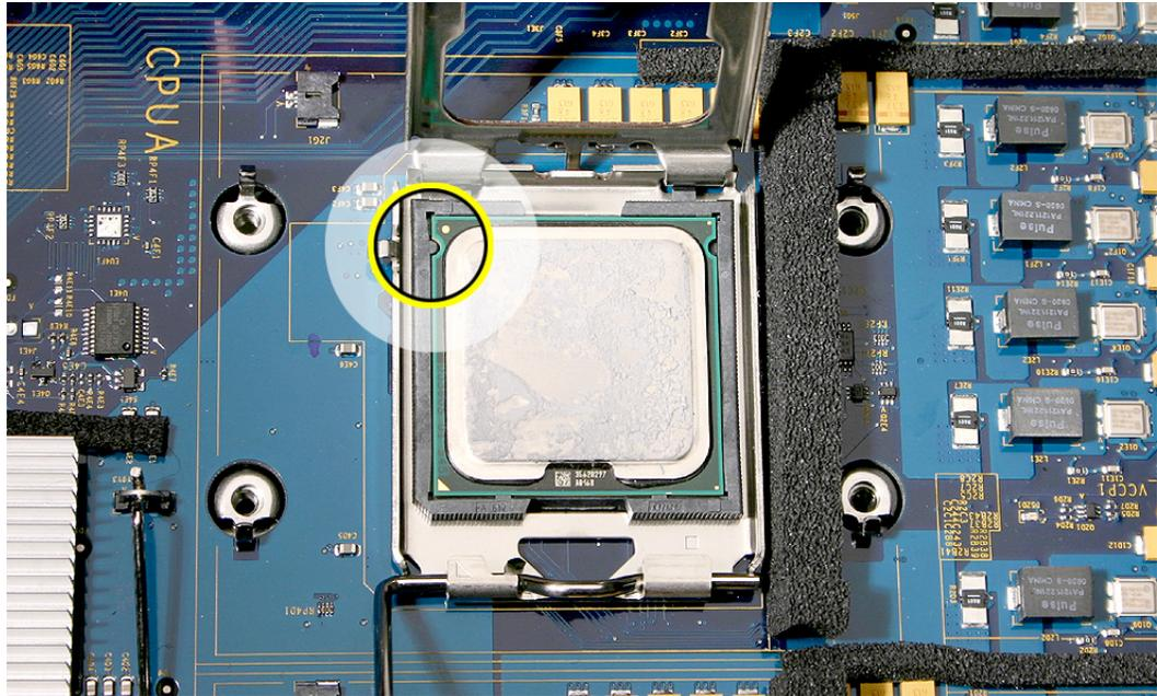
8. Rotate the top of the holder to the closed position.
