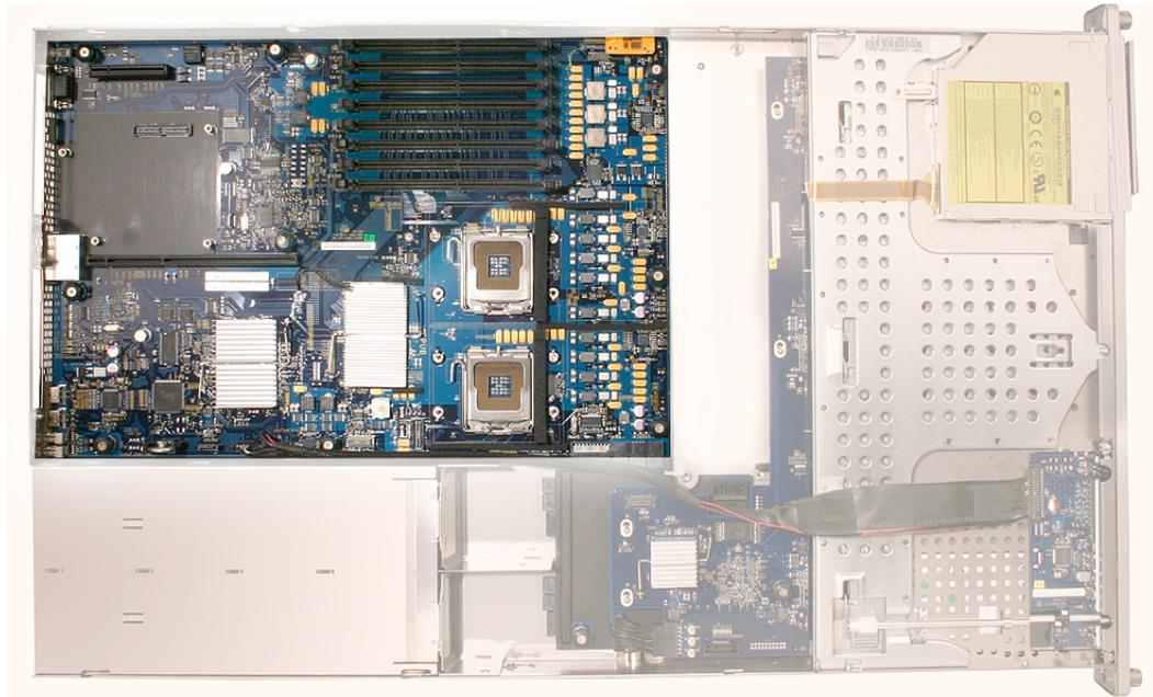
**Caution:** Although the logic boards for Xserve (Late 2006) and Xserve (Early 2008) are a similar size, do not install an older logic board in the Xserve (Early 2008) server.
