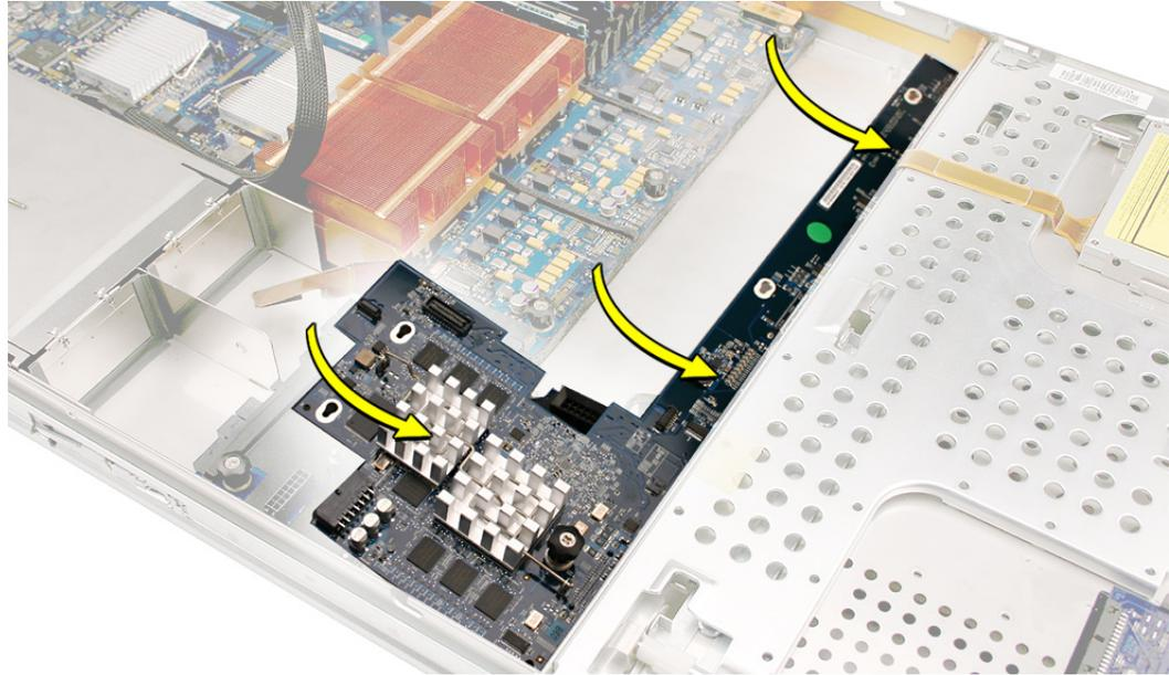
Then rotate the Xserve RAID Card downward and over the four mushroom-shaped standoffs. Finally, slide the card in the direction of the arrow shown to fully seat the card in the enclosure.
