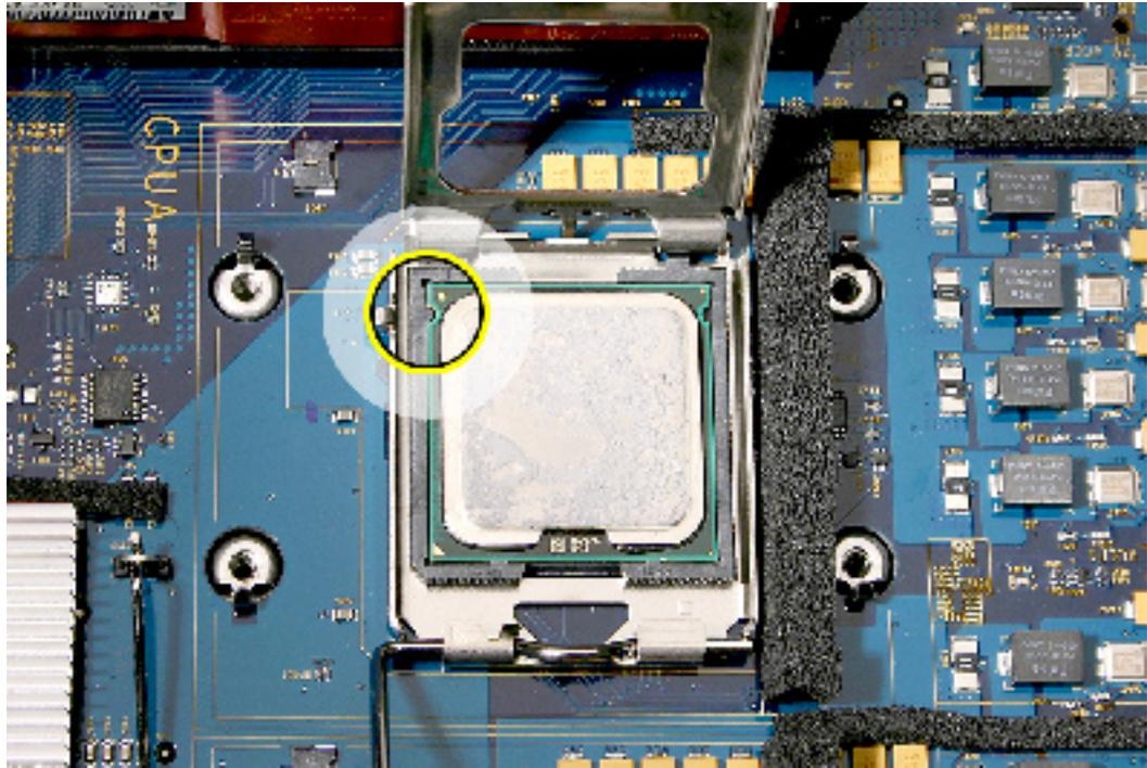
4. Rotate the top of the holder to the closed position.
