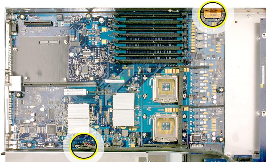
4. Loosen the single thumbscrew on the power distribution board and slide the board away from and out of the connector on the logic board.
