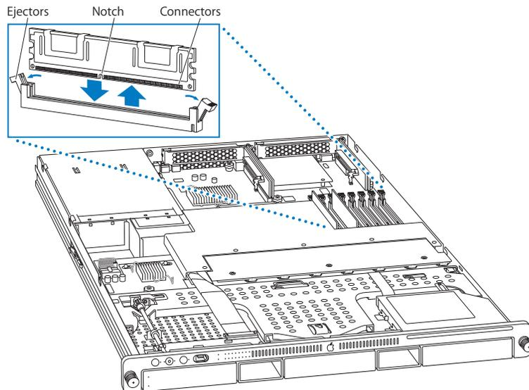
**Warning:** When removing or installing the DIMM, handle it only by the edges. Do not touch its connectors. Lift the DIMM straight up from the connector to remove it, and insert it straight down into the connector to install it. Do not rock the DIMM from side to side.
