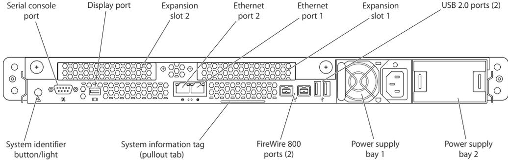
Note: The rear panel of the Xserve (Early 2008) and Xserve (Late 2006) model is identical to the image above except you might notice differences if a power supply blank is installed or one or more expansion cards are installed.
